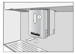
■ Push the main dispenser down completely ① and remove the stainless steel cover by pulling it off towards you ②.
